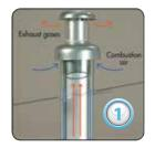
Sealed Combustion Appliance. The innovative "pipe-inside-a-pipe" roof jack, vents combustion gases while bringing air from outdoors to the burner, thereby producing a higher level of efficiency and safety.
