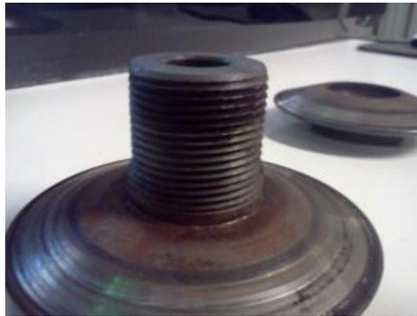
The two halves of an adjustable sheave
