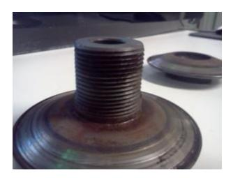
The two halves of an adjustable sheave
