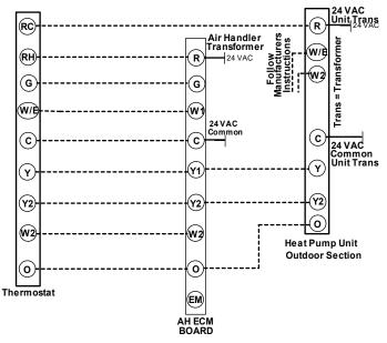
Figure 30: Typical Two Stage Heat with Two Stage Package Heat Pump
