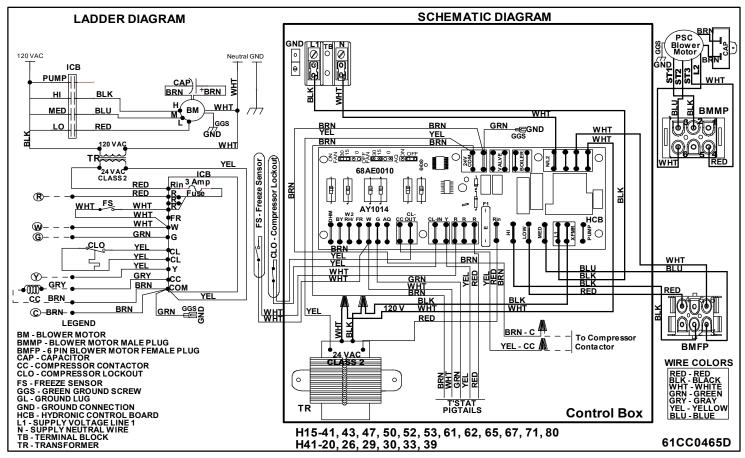
Figure 40 H40/H41/H14/H15/CWA4-HW Hydronic Heat w/out Pump W/Freeze Stat and CLO – PSC Blower Motor
