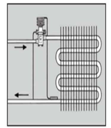
Figure 13: TXV Sensing Bulb Location
