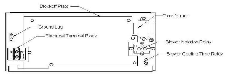
Figure 18: Component Locations - No Heat Control Box
