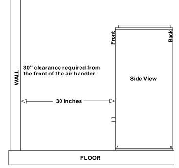
Figure 5: Clearance – Access for Service
