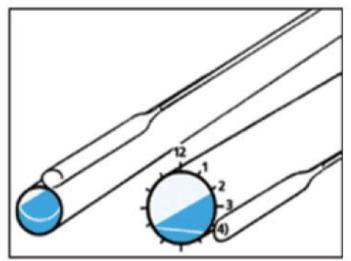
Figure 12: The TXV Bulb Best Placement
