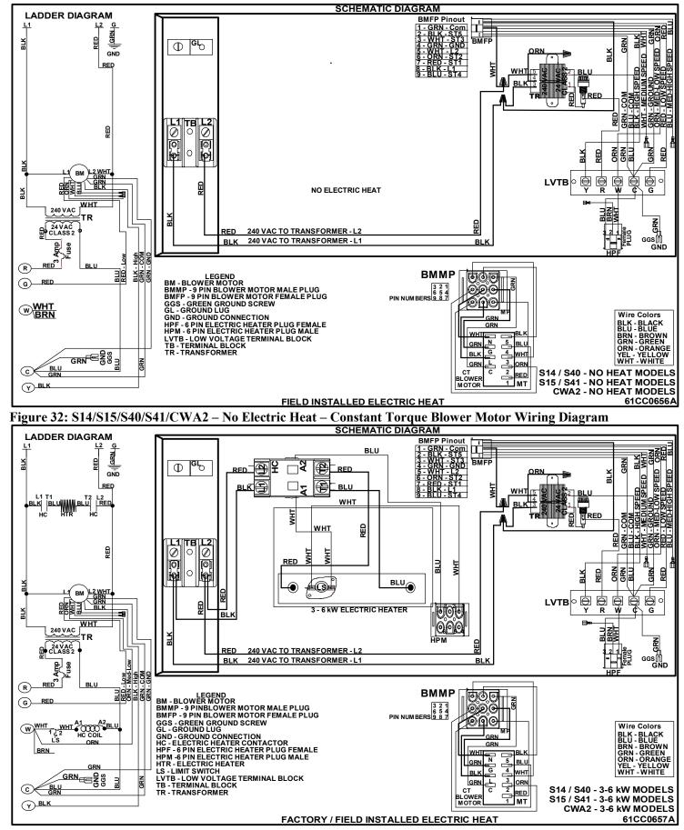
Figure 33: S14/S15/S40/S41/CWA2 – 3kW - 6kW Electric Heat. – Constant Torque Blower Motor Wiring Diagram
