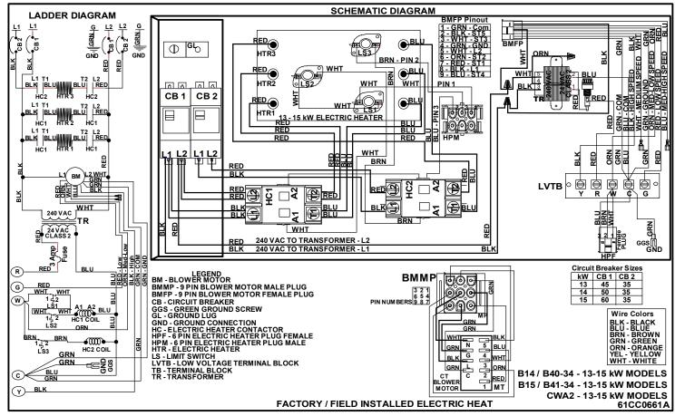
Figure 37 B14/B15/B40-34/B41-34/CWA2 13 kW - 15kW Electric Heat – Constant Torque Blower Motor 501 TERMINAL RD FORT WORTH, TEXAS 76106
