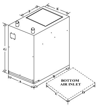
Figure 4: H40/H14 DIMENSIONAL DATA NO COOLING WITH OR WITHOUT ELECTRIC HEAT
