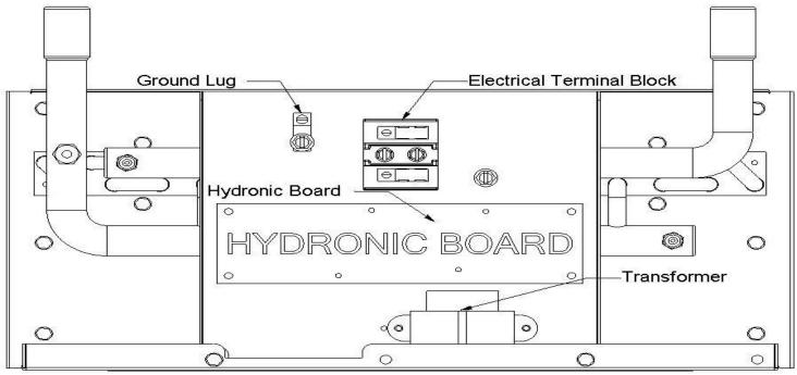
Figure 19: Component Locations – Hydronic Heat Control Box
