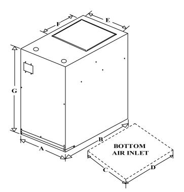
Figure 3: B-S40/B-S14 DIMENSIONAL DATA NO COOLING WITH OR WITHOUT ELECTRIC HEAT
