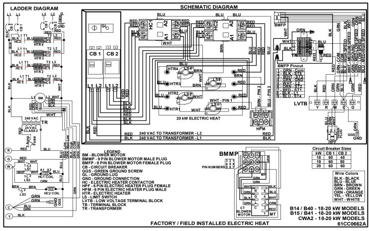
Figure 38 B14/B15/B40/B41/CWA2 18 kW - 20kW Electric Heat - Constant Torque Blower Motor
