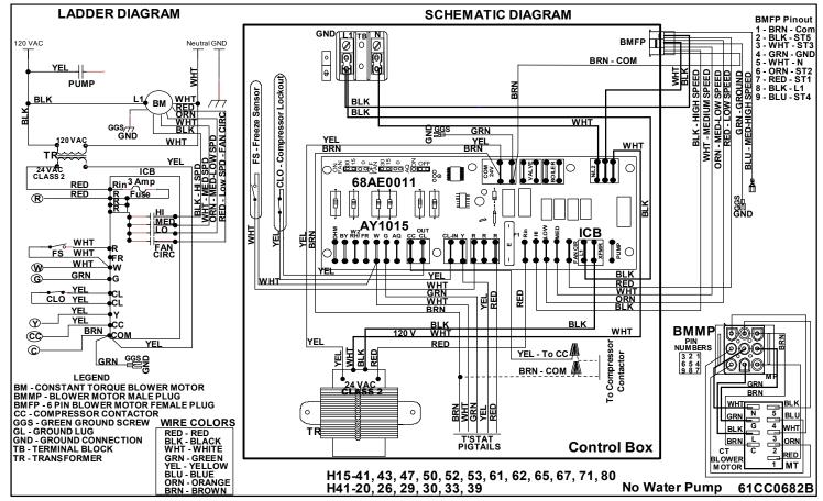
Figure 41 H40/H41/H14/H15/CWA4-HW Hydronic Heat w/out Pump W/Freeze Stat and CLO – C.T. Blower Motor 501 TERMINAL RD FORT WORTH. TEXAS 76106
