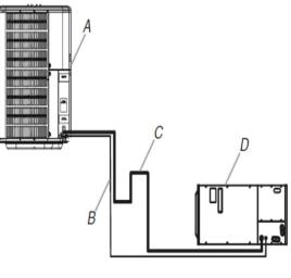
A. Condensing unit B. Liquid line
