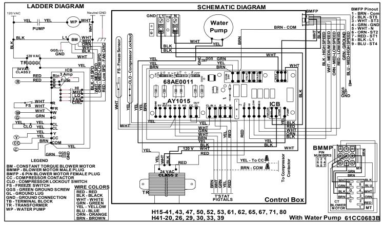
Figure 42 H40/H41/H14/H15/CWA4-HW Hydronic Heat with Pump W/Freeze Stat and CLO – C.T. Blower Motor
