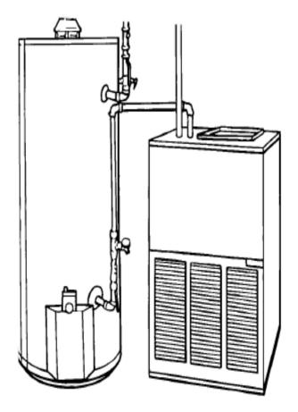
Figure 9: Typical Hot Water Tank Connections
