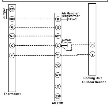
Figure 23: Typical Single Stage Heat with Single Stage Split System Cooling
