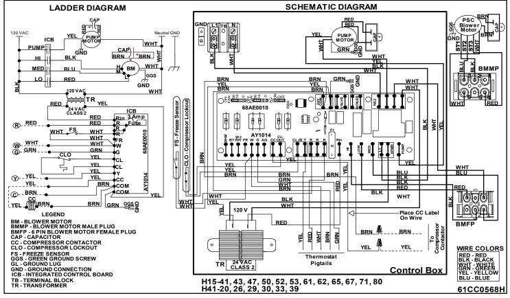
Figure 43 H40/H41/H14/H15/CWA4-HW Hydronic Heat with Pump, Freeze Stat and CLO – PSC Blower Motor
