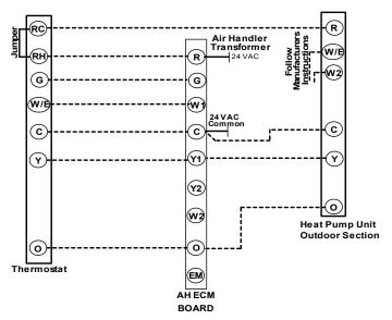
Figure 25: Typical Single Stage Heat with Single Stage Split System Heat Pump
