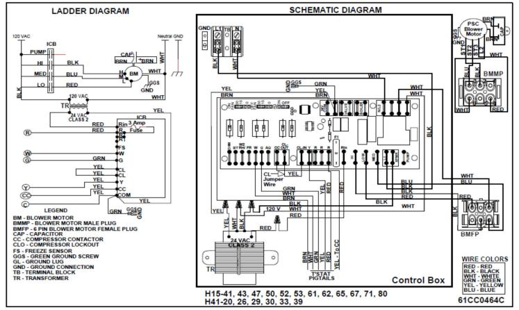
Figure 39 H40/H41/H14/H15/CWA4-HW Hydronic Heat with Pump, Freeze Stat and CLO – PSC Blower Motor
