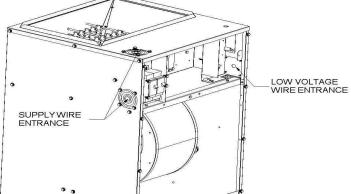
Figure 22: Supply Wire Knockout and Low Voltage Thermostat Wire Entrance Locations
