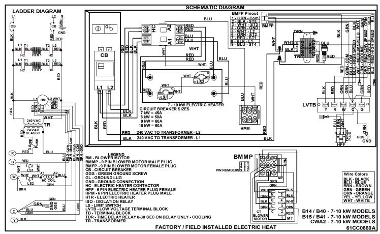
Figure 36 B14/B15/B40/B41/CWA2 7kW – 10kW Electric Heat – Constant Torque Blower Motor Wiring Diagram
