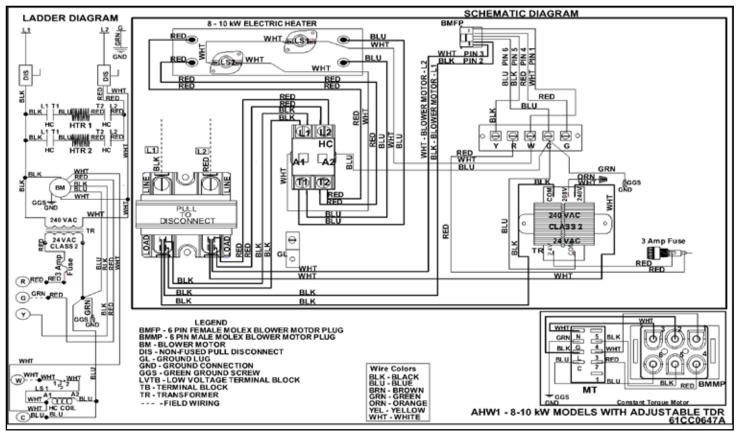
Figure 39: 8 kW and 10 kW Electric Heat Wiring Diagram
