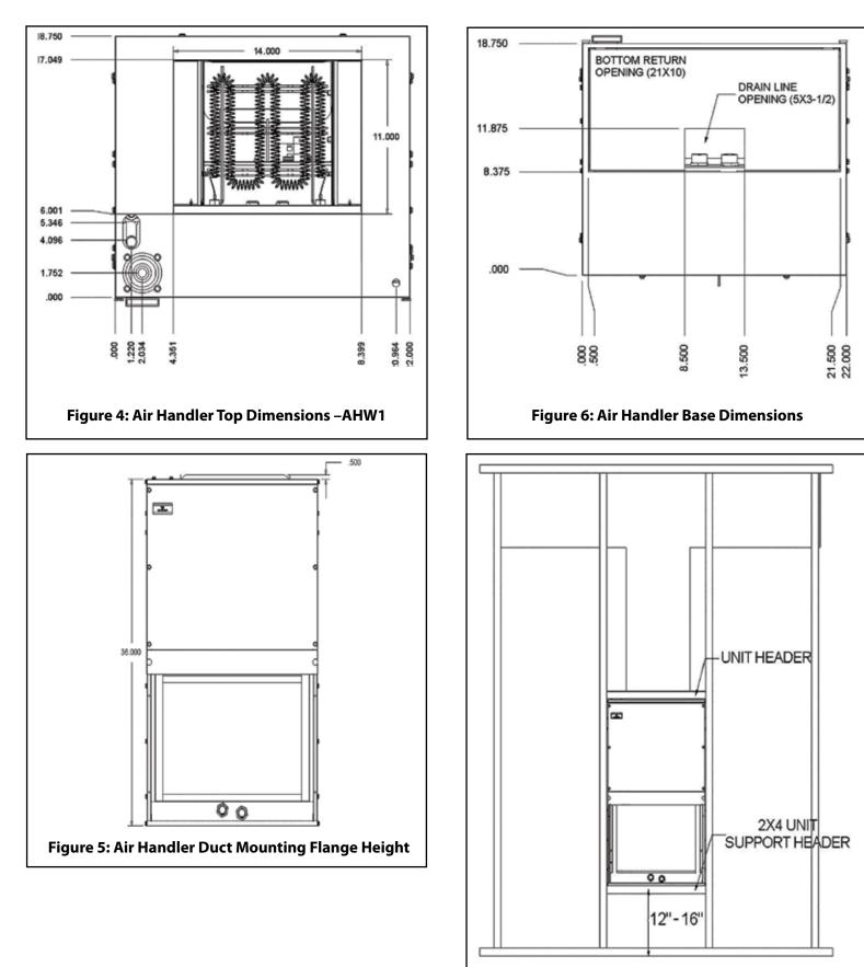
Figure 7: Typical Wall Mount Installation
