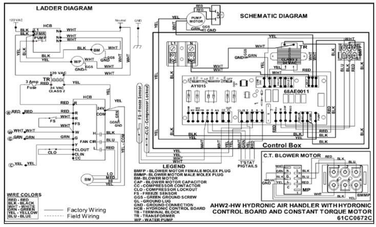
Figure 40: Hydronic Heat Wiring Diagram
