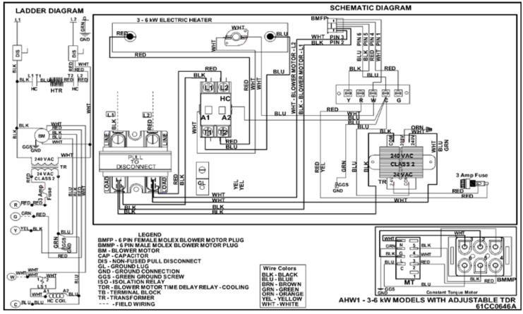
Figure 38: 3 kW, 5 kW and 6 kW Electric Heat Wiring Diagram
