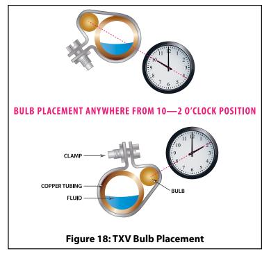
The best location for the TXV sensing bulb is on a horizontal section of the suction line tube and positioned between 10 o'clock and 2 o'clock on the tube. (See Figures 8 and 9).
