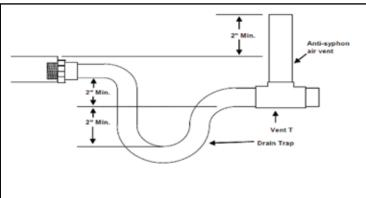
Figure 23: Typical Condensate Trap
