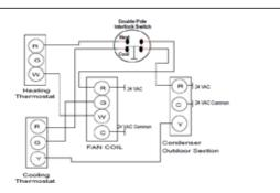
Figure 26: Heat/Cool Thermostat Connections - Separate Thermostats & Separate Transformers in Air Handler and Outdoor Unit
