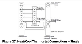
Thermostat & Separate Transformers in Air Handler & Outdoor Unit
