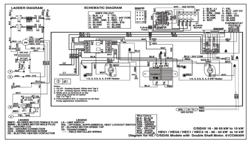
Figure 33: HE\*1/HE\*3 – 03kW to 10kW Electric Heat – Constant Torque Motor
