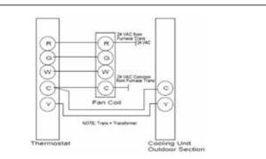
Figure 28: Heat/Cool Thermostat Connections - Single Thermostat & Single Transformer in Air Handler
