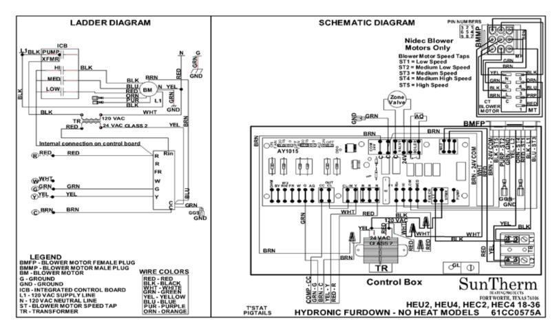
Figure 34: HE\*2/HE\*4 – No Hydronic Heat – Constant Torque Motor
