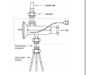
Figure 14: Typical TXV Connections
