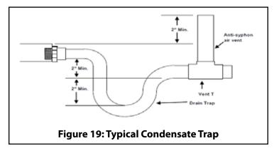
The cooling DX coil condensate drain pan has a 3/4" NPT male primary connection on each side and one 3/4" NPT male secondary connection on one side. The two primary drain connections may need to be tied together before the trap to allow the drain pan to fully drain because of the high air velocity across the coil. Refer to Figure 20 for options for the primary drain connections.
