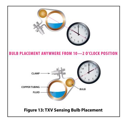
The best location for the TXV sensing bulb is on a horizontal section of the suction line tube and positioned between 10 o'clock and 2 o'clock on the tube. (See Figures 7 and 8).
