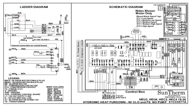
Figure 36: HE\*2/HE\*4 – Hydronic Heat No Pump – Constant Torque Motor
