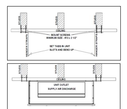
Figure 10: Air Handler Mounting
