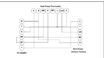
Figure 29: Heat Pump Thermostat Connections - Single Thermostat & Single Transformer in Air Handler
