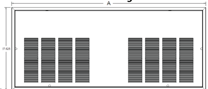
Figure 4: HEC Dimensions - Front
