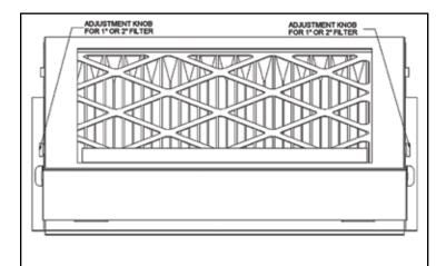
Note: Adjustment knobs are on each side.
