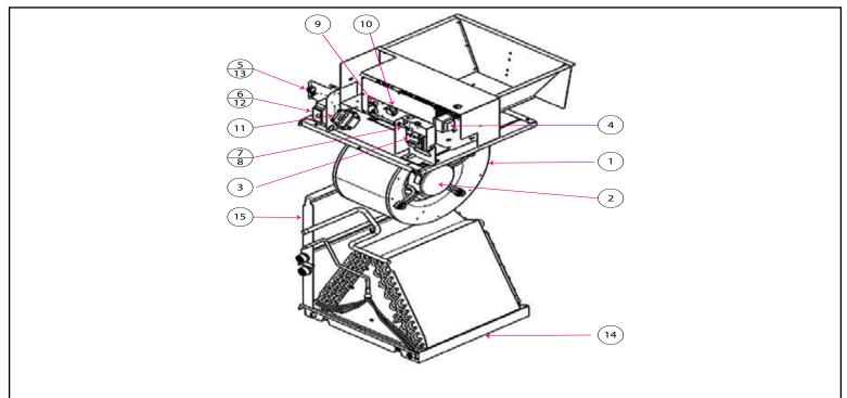
Figure 22: MS 18, 24 Electric Heat Air Handler Replacement Parts Schematic
