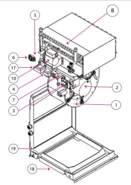
Figure 27: MS 37, 42, 48, 60, 72 Hydronic Heat Air Handler Replacement Parts Schematic
