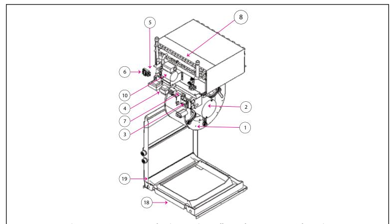
Figure 26: MS 25, 30, 36 Hydronic Heat Air Handler Replacement Parts Schematic
