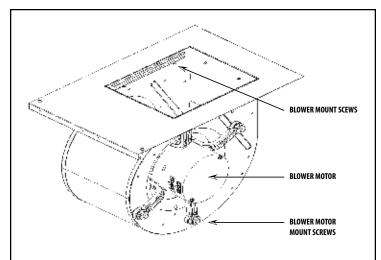
**Figure 17: Blower Mounting Plate Screw Locations**
