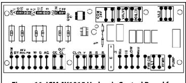
Figure 11: ICM AY1015 Hydronic Control Board for Constant Torque and ECM Motors
