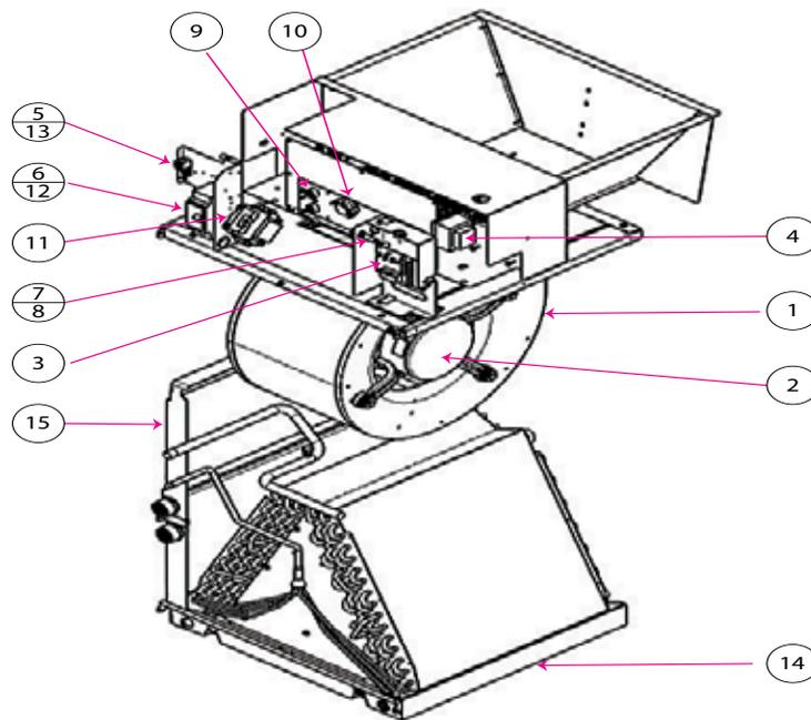
**Figure 22: MS 18, 24 Electric Heat Air Handler Replacement Parts Schematic**
