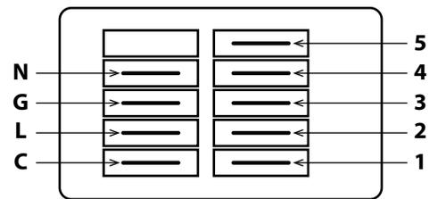
**Figure 15: Constant Torque Motor Terminals**
