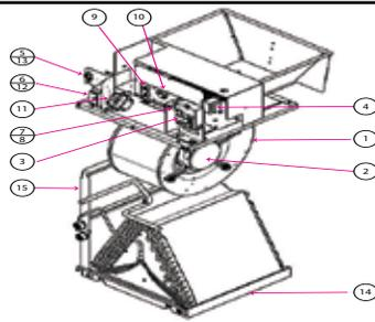
**Figure 24: MS 37, 42, 48, 60, 72 Electric Heat Air Handler Replacement Parts Schematic**
