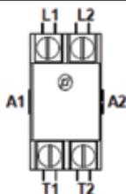
**Figure 16: Heater Contactor Terminals**
