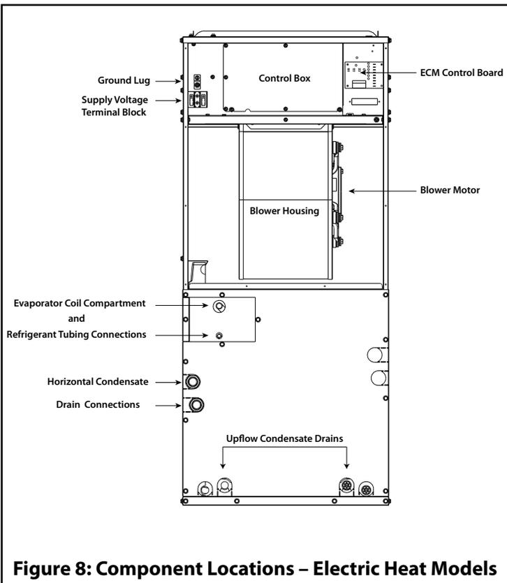
Figure 8: Component Locations – Electric Heat Models
