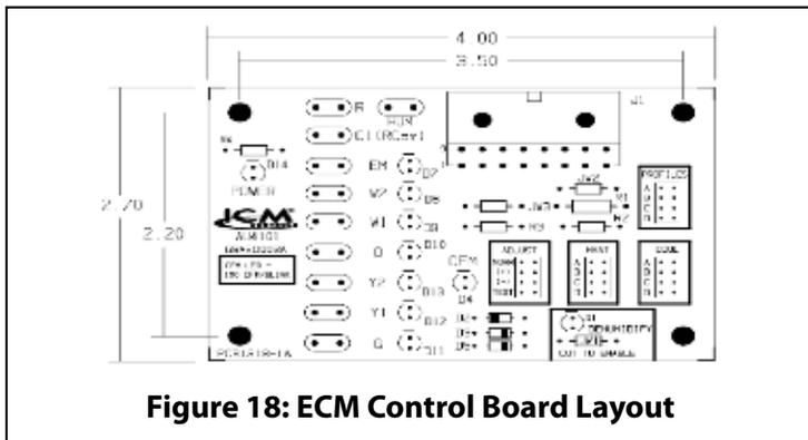
Figure 18: ECM Control Board Layout
