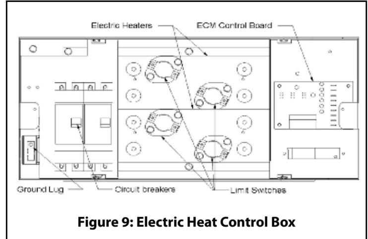
Figure 9: Electric Heat Control Box
