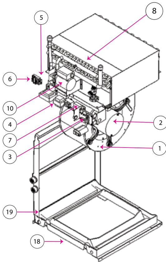
**Figure 26: MS 25, 30, 36 Hydronic Heat Air Handler Replacement Parts Schematic**
