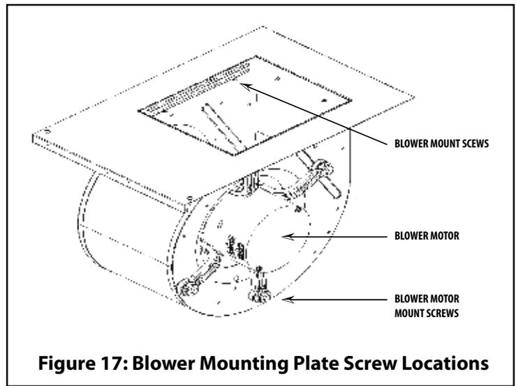
**Figure 17: Blower Mounting Plate Screw Locations**
