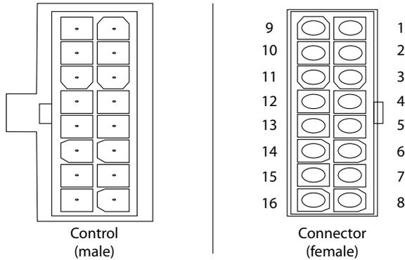
**Figure 14: ECM Motor Control Pin Positions**
