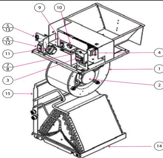
**Figure 23: MS 25, 30, 36 Electric Heat Air Handler Replacement Parts Schematic**
