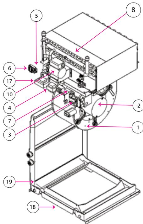
**Figure 27: MS 37, 42, 48, 60, 72 Hydronic Heat Air Handler Replacement Parts Schematic**
