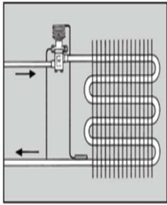
**Figure 19: TXV Sensing Bulb Location**
