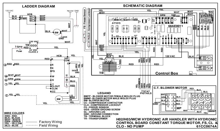
Figure 49 H02 / H03 Hydronic Heat - No Pump, With CLO and Freeze Stat – Constant Torque Blower Motor
