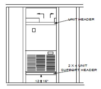
**Figure 9: Typical Wall Mount Installation**
