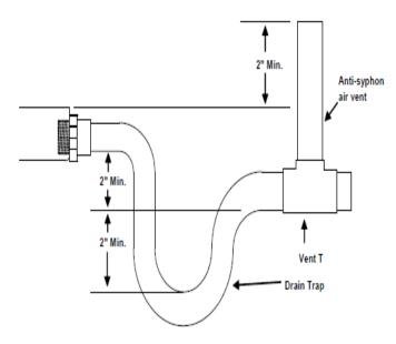
Figure 22: Typical Condensate Trap
