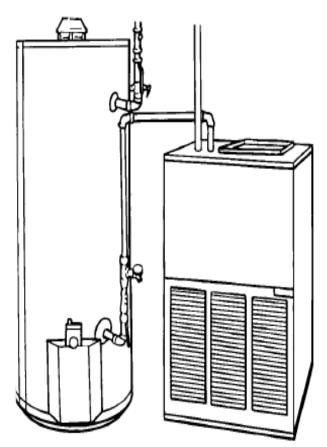
**Figure 15: Typical Hot Water Tank Connections**
