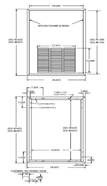
**Figure 12: Optional Wall Panel Door Dimensions**
