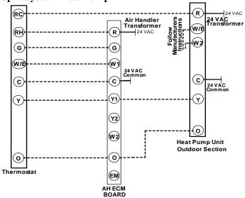
Figure 32: Typical Single Stage Heat with Single Stage Package Heat Pump Unit
