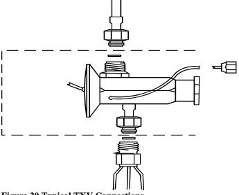
Figure 20 Typical TXV Connections
