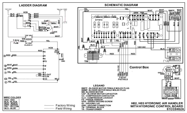
Figure 47 H02 / H03 Hydronic Heat - No Pump, CLO or Freeze Stat – PSC Blower Motor
