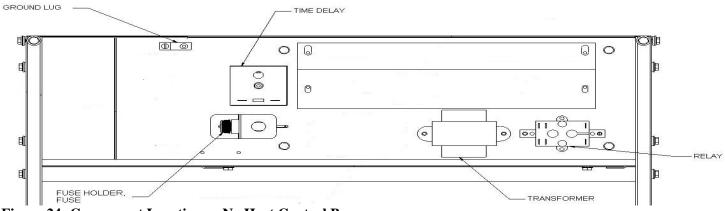
Figure 24: Component Locations - No Heat Control Box
