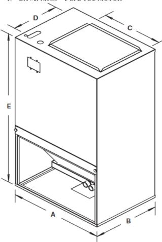
Figure 1: B-S02/B-S03/WCW DIMENSIONAL DATA DX COOLING WITH OR WITHOUT ELECTRIC HEAT
