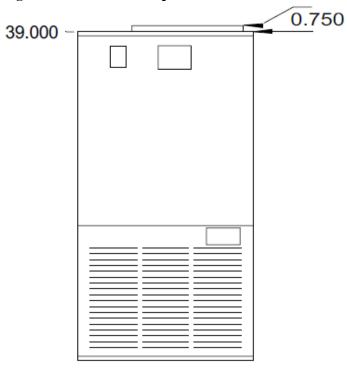
**Figure 8: Air Handler Supply Duct Mounting Flange Dimensions**
