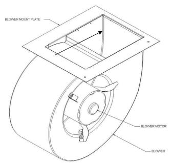
Figure 38: Blower Assembly and Blower Deck
