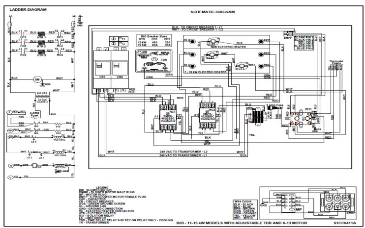
Figure 44 B03 12kW – 15kW Electric Heat – Constant Torque Blower Motor
