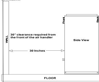
Figure 3: Clearance – Access for Service
