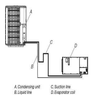
Figure 17 Evaporator Below Condenser Piping SPECIAL INSTRUCTIONS FOR COILS WITH THERMAL EXPANSION VALVES (TXV)
