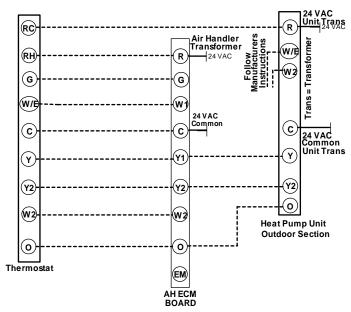
Figure 36: Typical Two Stage Heat with Two Stage Package Heat Pump
