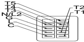
**Figure 37: Constant Torque Motor Terminals**
