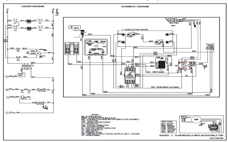
Figure 42 S02/S03 7kW – 10kW Electric Heat – PSC Blower Motor Wiring Diagram
