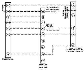
Figure 31: Typical Single Stage Heat with Single Stage Split System Heat Pump
