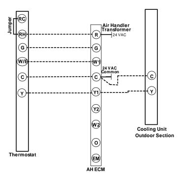
Figure 29: Typical Single Stage Heat with Single Stage Split System Cooling
