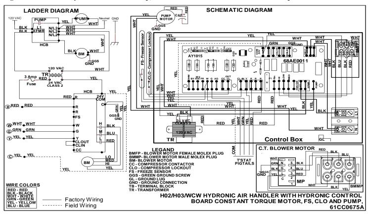
Figure 50 H02 / H03 Hydronic Heat - With Pump, CLO and Freeze Stat - Constant Torque Blower Motor
