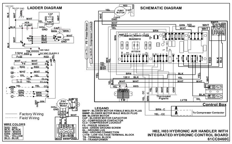
Figure 45 H02 / H03 Hydronic Heat - With Pump, CLO and Freeze Stat - PSC Blower Motor
