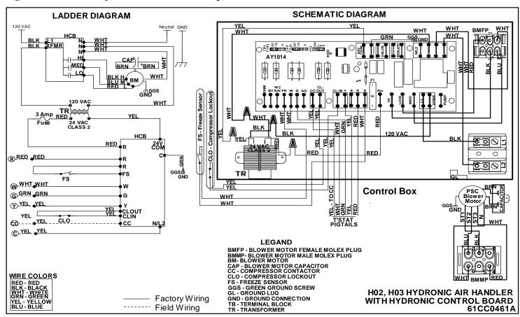
Figure 46 H02 / H03 Hydronic Heat - No Pump - With CLO and Freeze Stat - PSC Blower Motor
