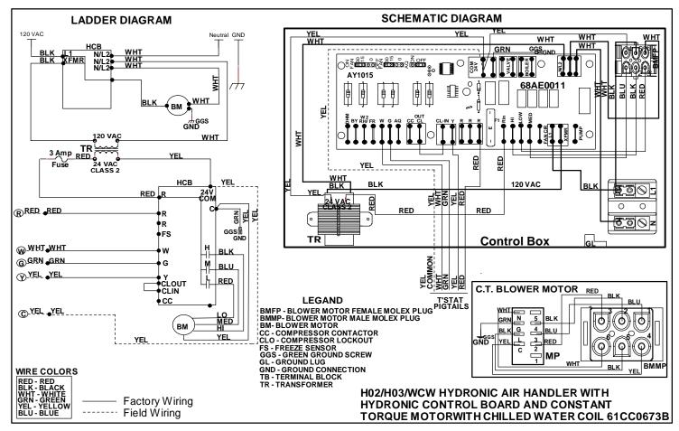
Figure 48 H02 / H03 Hydronic Heat - No Pump, CLO or Freeze Stat - Constant Torque Blower Motor
