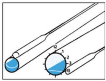
Figure 18: The TXV Bulb Best Placement
