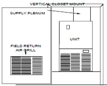
**Figure 10: Typical Wall Mount Installation with Wall Panel Door**
