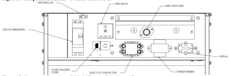
Figure 25: Component Locations – B Model Electric Heat Control Box
