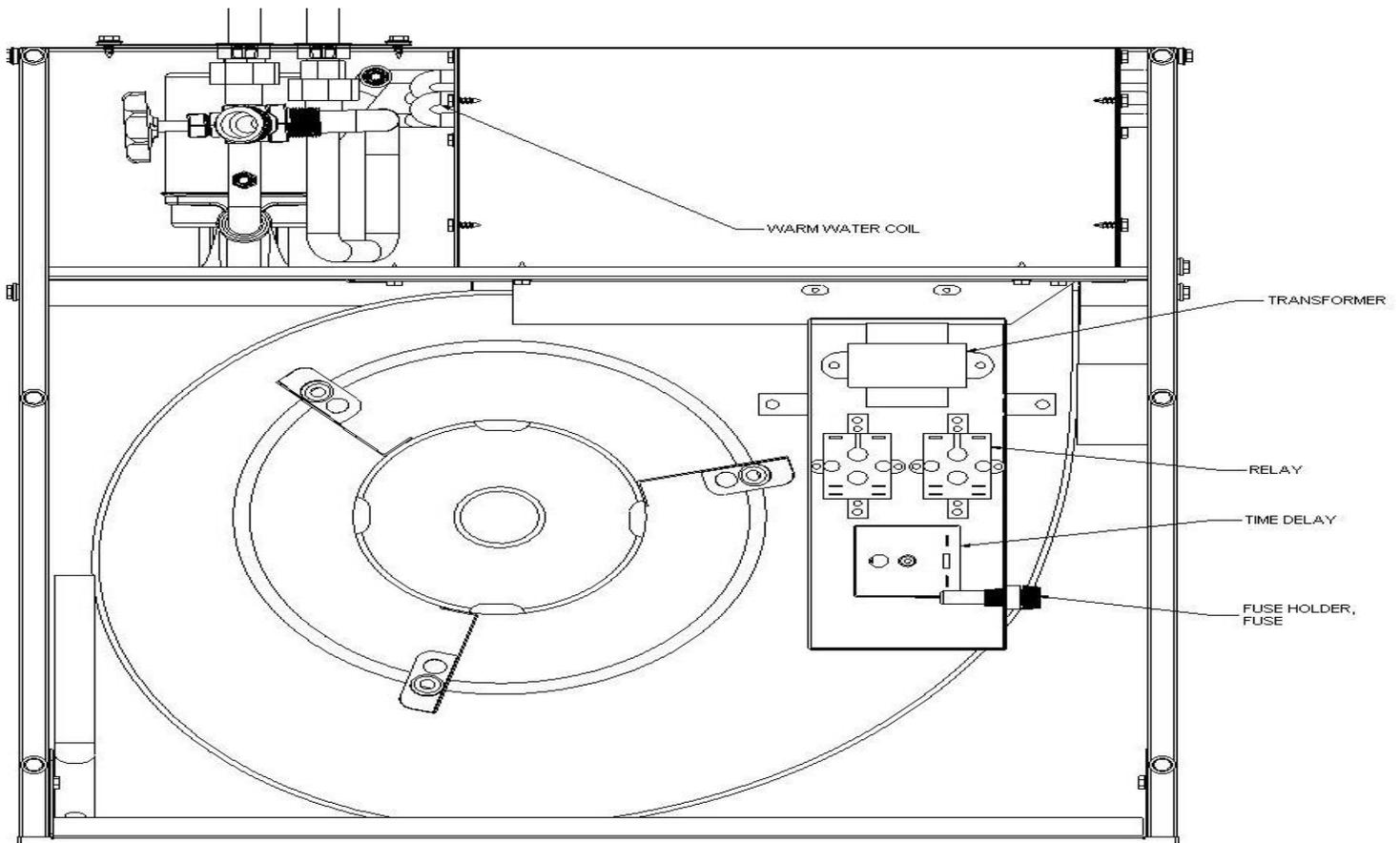
**Figure 26: Component Locations – Hydronic Heat Control Box**
