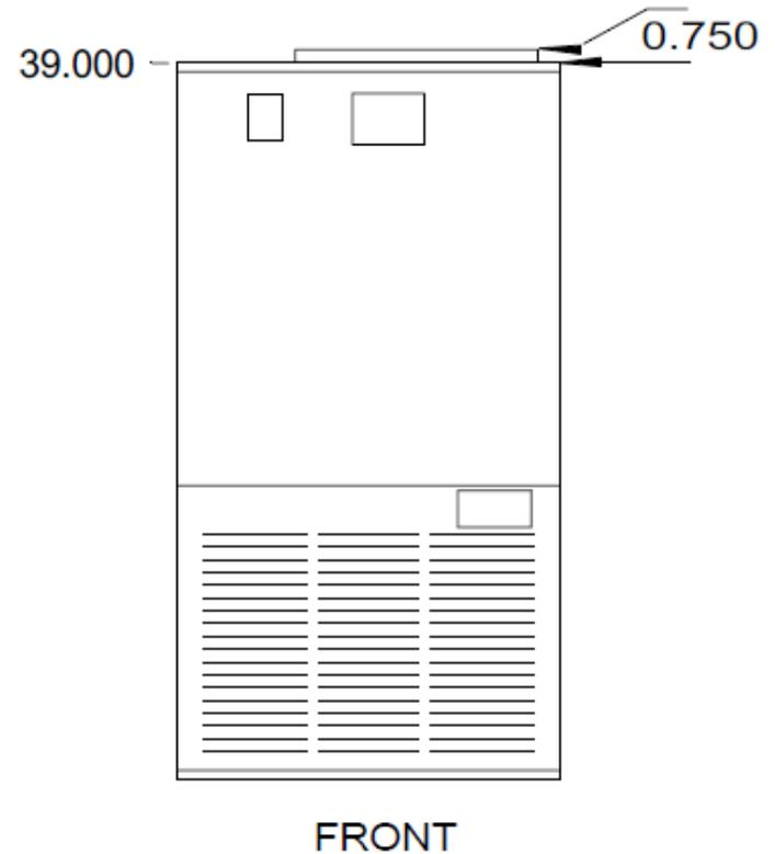
**Figure 8: Air Handler Supply Duct Mounting Flange Dimensions**
