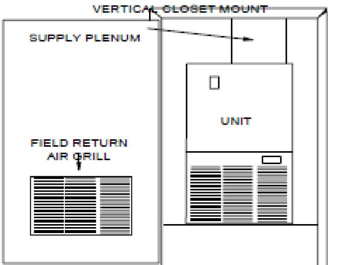
Figure 10: Typical Wall Mount Installation with Wall Panel Door
