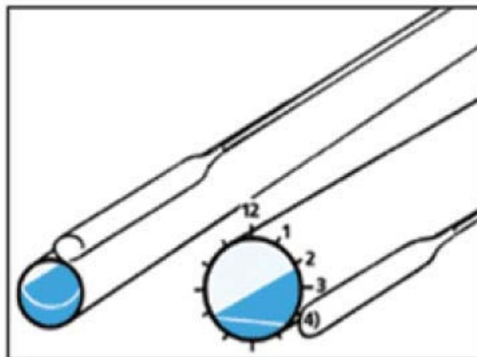
**Figure 18: The TXV Bulb Best Placement**
