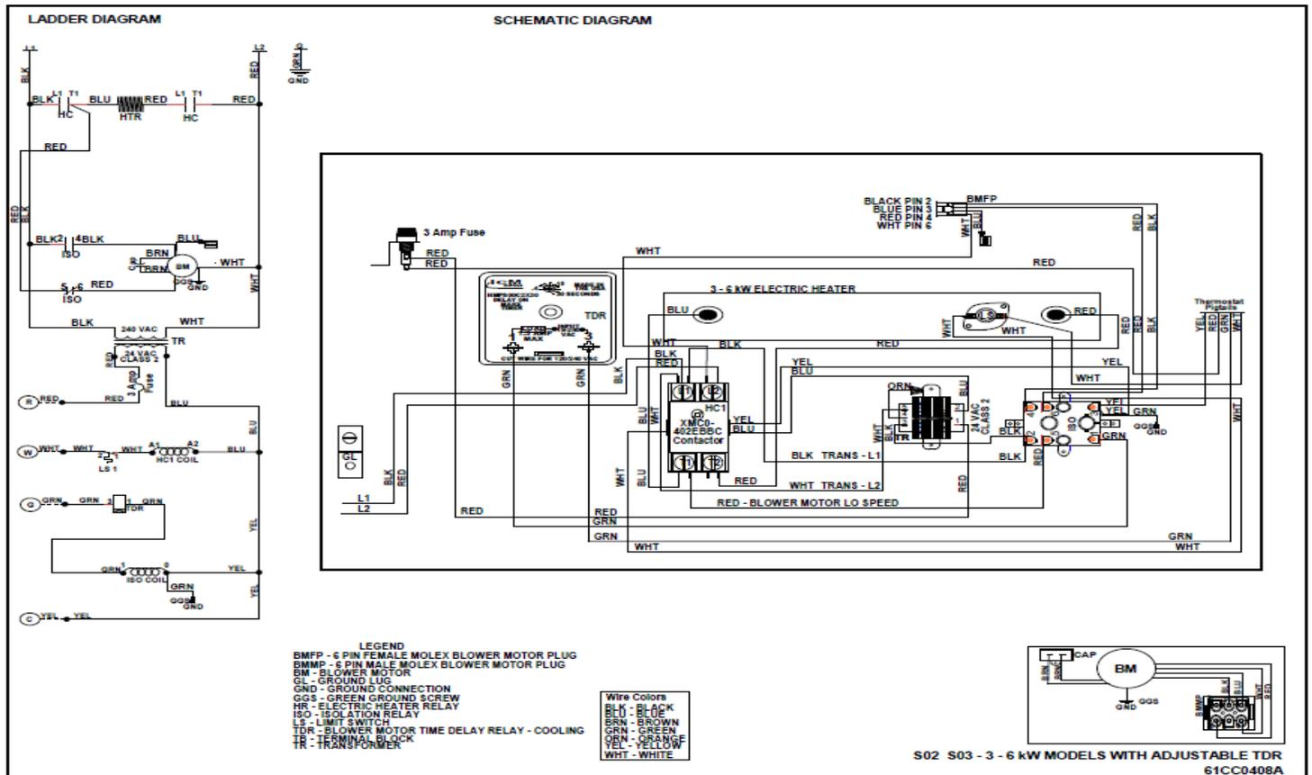
Figure 40: S02/S03 – 3kW - 6kW Electric Heat. – PSC Blower Motor Wiring Diagram
