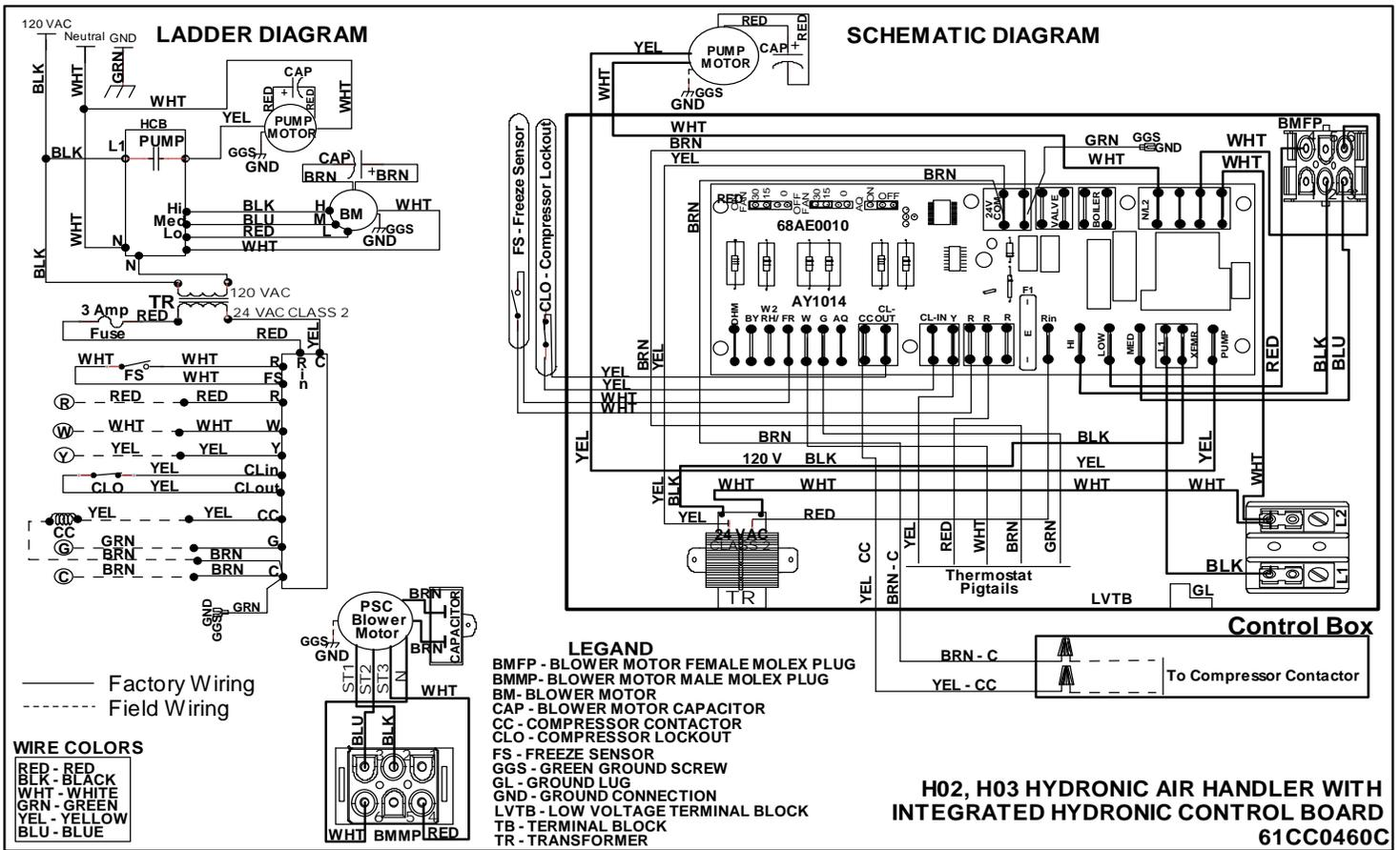
Figure 45 H02 / H03 Hydronic Heat - With Pump, CLO and Freeze Stat – PSC Blower Motor
