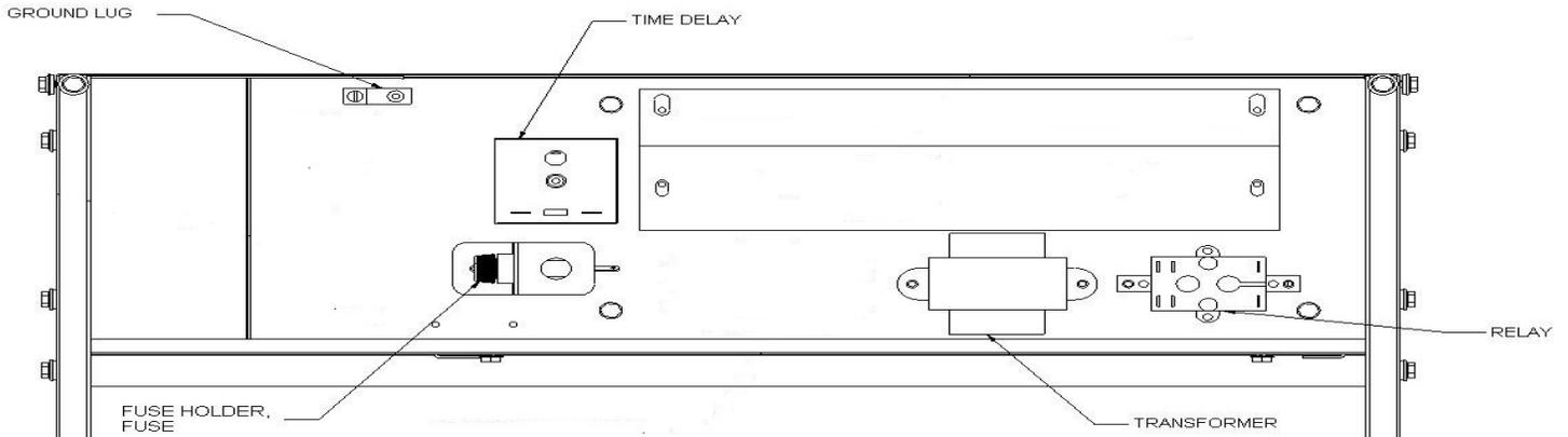
**Figure 24: Component Locations – No Heat Control Box**
