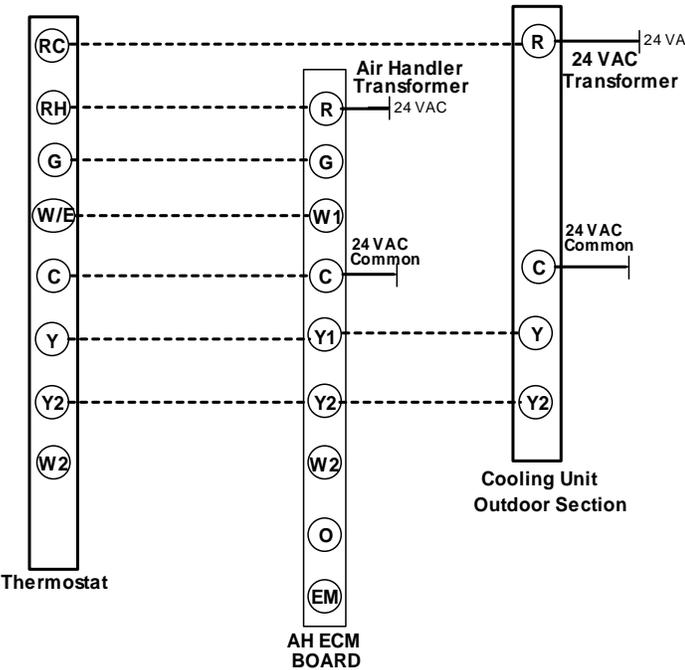
**Figure 34: Typical Single Stage Heat with Two Stage Package Cooling Unit**
