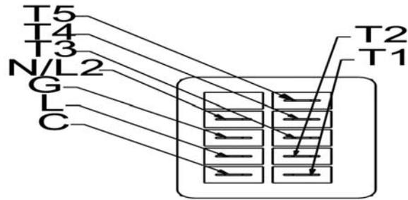
**Figure 37: Constant Torque Motor Terminals**
