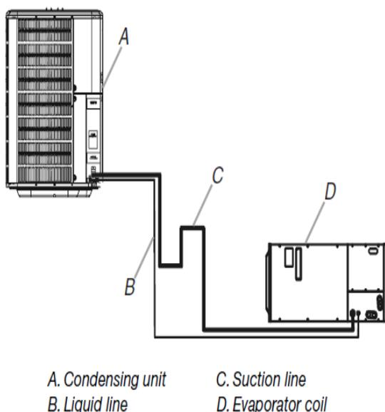
**Figure 17 Evaporator Below Condenser Piping**
