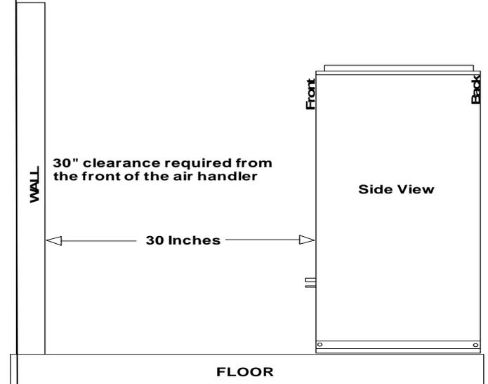
Figure 3: Clearance – Access for Service
