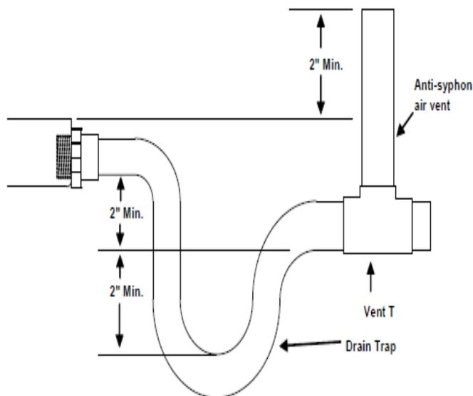
Figure 22: Typical Condensate Trap
