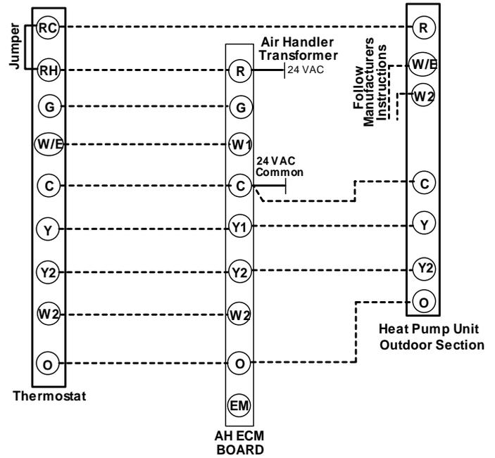
**Figure 35: Typical Two Stage Heating with Two Stage Split System Heat Pump**
