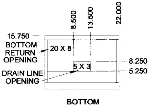
**Figure 6: Air Handler Base Dimensions**
